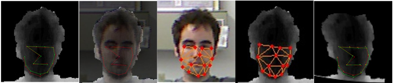
Figure 1: Far left: candidate registration points – RGB image points shown in green and depth image points shown in red. Left middle: transparent overlay of RGB and depth images with depth window border. Center: active shape model fitted to RGB image. Right middle: active shape model fitted to depth image. Far right: registration results after deformation – RGB points in green and depth points in red.
